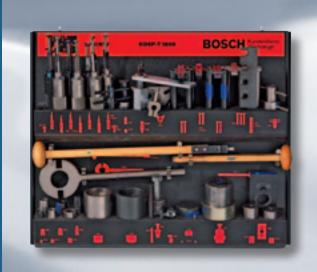
Repair of in-line fuel-injection pumps of model series PE(S) ..MW.. S1 (8 mm stroke) ..S100 (10 mm stroke) and ..S1500, **without** controller, charge-pressuredependent full-load stop (LDA) and timing device
