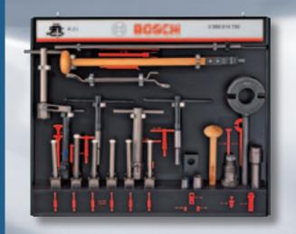
Repair of in-line fuel-injection pumps of the model series PE(S)..A..D/S 1000, -/S 2000, -/3000 **without** controller, charge-pressure-dependent full-load stop (LDA) and timing device
