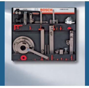
**Tool set** for repair of electronically controlled in-line fuel-injection pumps (EDC) of sizes R, (M)
