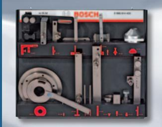
Repair of electronically controlled in-line fuel-injection pumps (EDC) of sizes H, R, (M)
