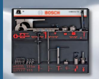
Repair of in-line fuel-injection pumps of model series PE(S) ..M.. with and without port-closing sensor system (FBG system), **without** controller, atmospheric-pressuredependent full-load stop (ADA) and timing device
