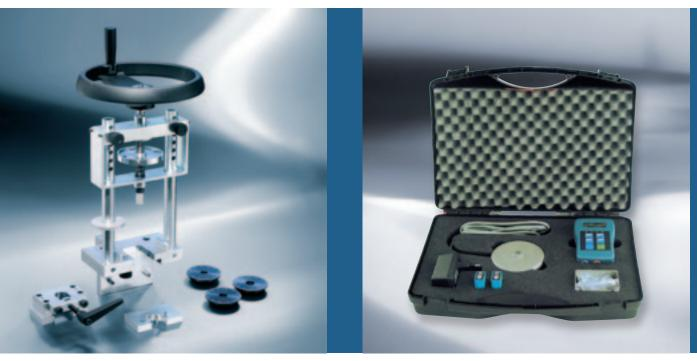
Assembly device for nozzle replacement
