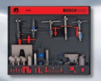
Repair of in-line fuel-injection pumps of the model series PE(S)..A..D/S 1000, -/S 2000, -/3000 **without** controller, charge-pressure-dependent full-load stop (LDA) and timing device
