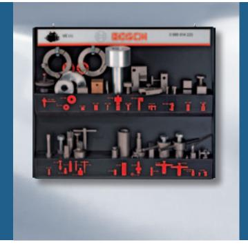
**Tool set** for repair of mechanically controlled distributor injection pumps (VE)
